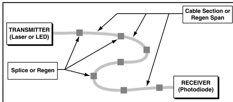
*Figure 1 - Typical Fiber Optic Transmission System*
