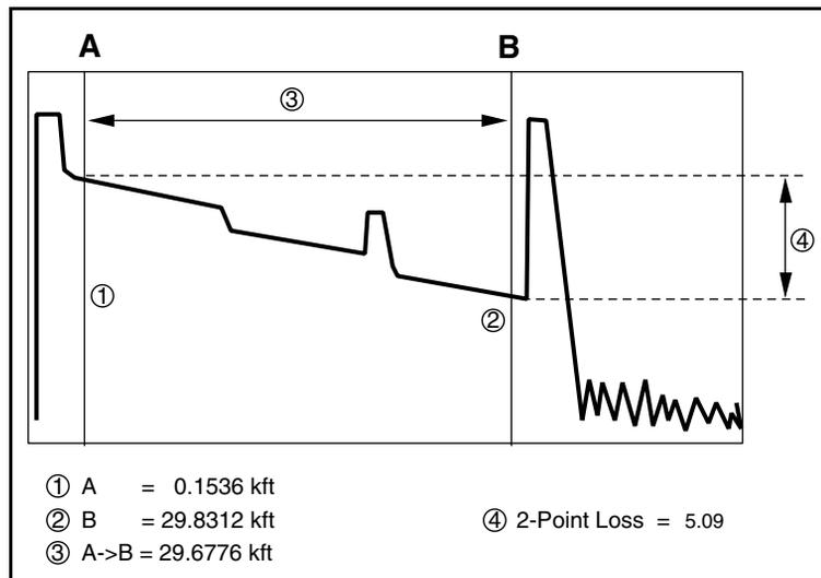
Figure 17 - OTDR Measurements Display
