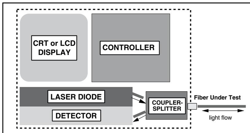
*Figure 4 - OTDR Block Diagram*
