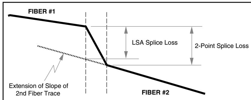
*Figure 18 - LSA vs. 2-Point Splice Loss*
