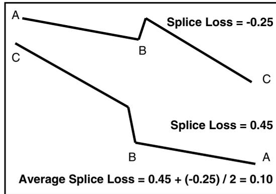
*Figure 20 - Treatment of Gain Splices*
