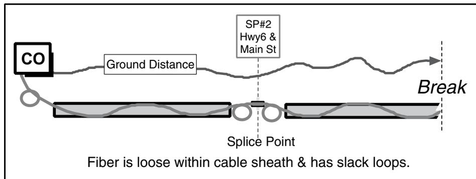
*Figure 14 - Fiber Distance Measurements*
